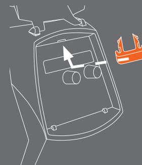
**6** EN When connecting a cooling circuit, observe the colour coding.
